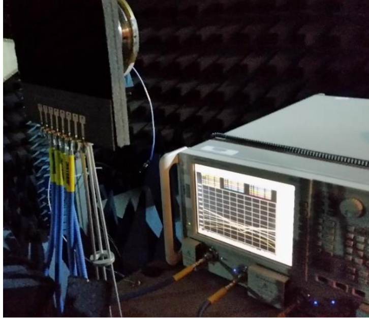
Figure 4.26 PNA-X and ULA setup in RMC's anechoic chamber
