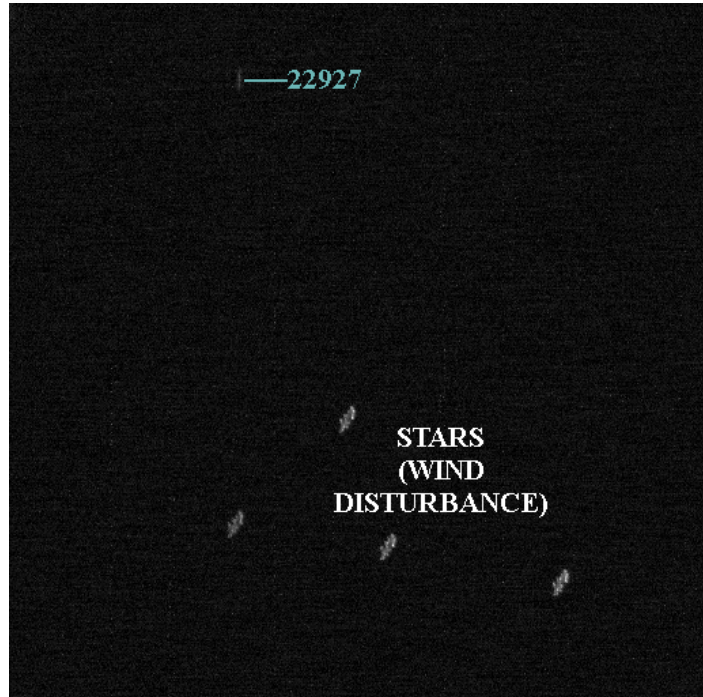
Figure 5.2: Image of 1-second Exposure Showing Unacceptable Star Distributions
