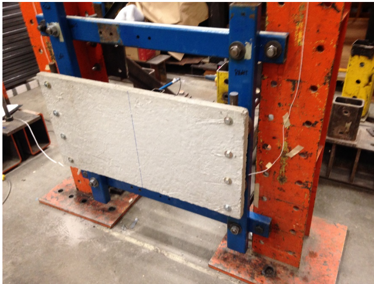
Figure 1-16 - Bolted connection of specimen to testing frame
