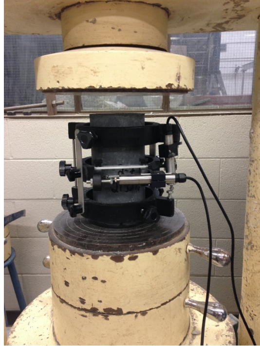
Figure 1-6 - Modulus of Elasticity Testing Setup
