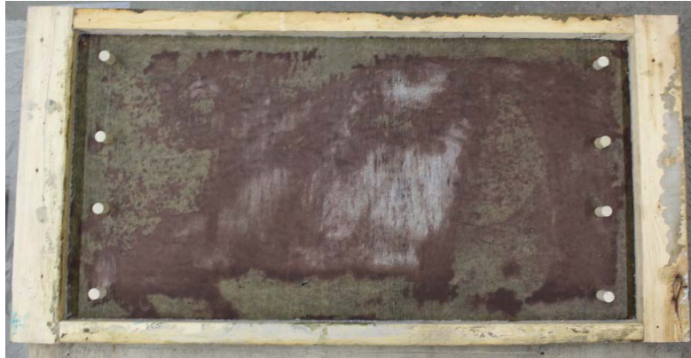
Figure 1-2 - Forms used to cast specimens
