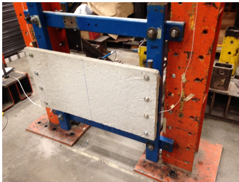
Figure 3-3 - Bolted connection of specimen to testing frame
