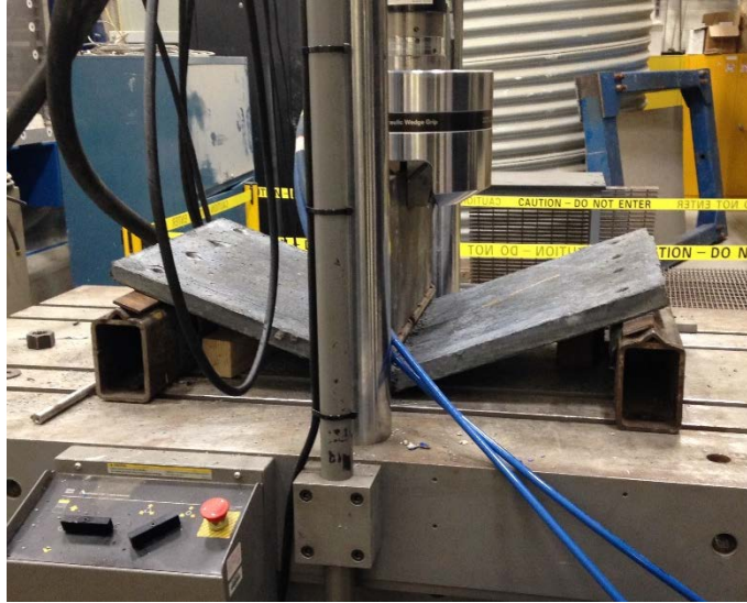
Figure 1-9 - Three-point flexural bending quasi-static testing set-up
