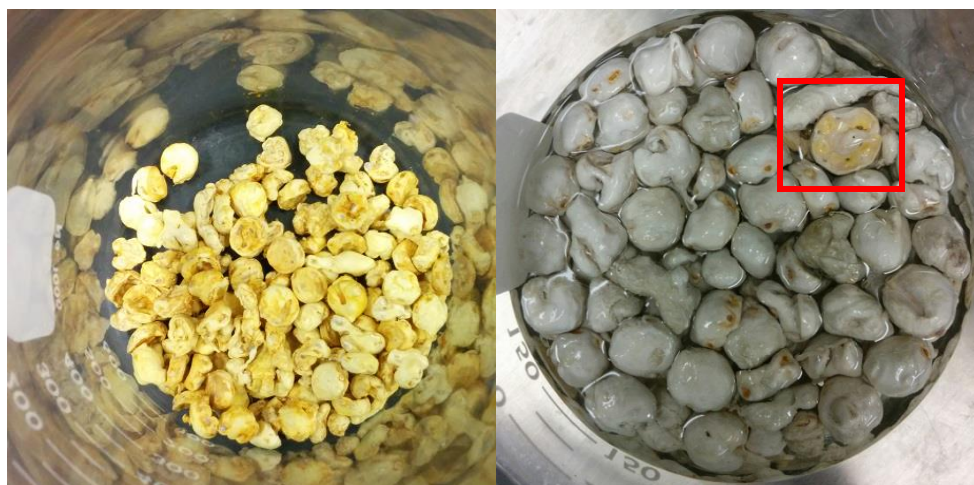
Figure 20: SPEEK pellets used as the catalyst. The left shows what they look like when dehydrated, and the right shows how they look when they absorb methanol.
