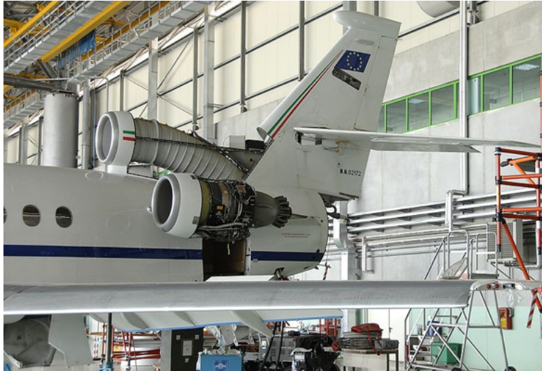
Figure 1.2: Section of Falcon 900EX showing S-duct [1]
