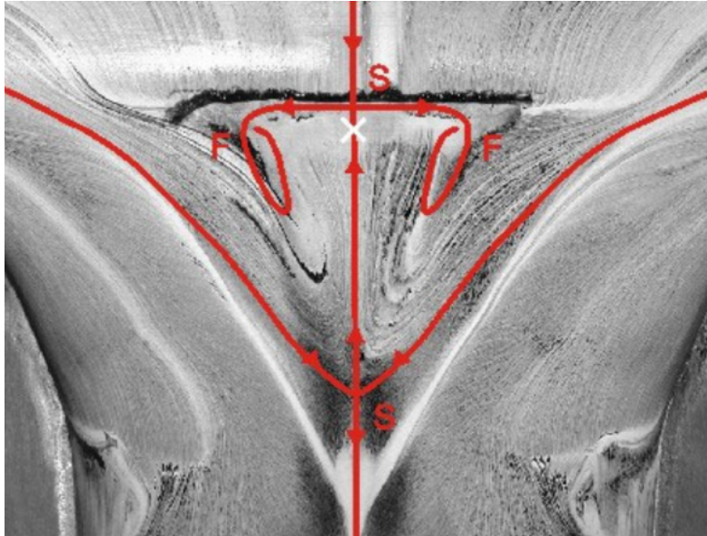
Figure 3.1: S-duct surface flow visualization in a region of reversing flow after an inner radius [14]
