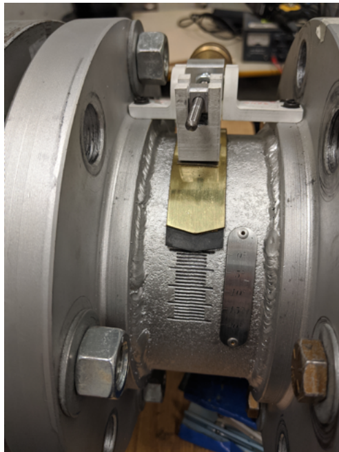
Figure 4.3: Iris valve used to set Mach number
