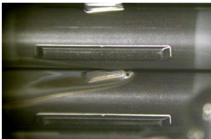
Figure 11. Fuel damage from debris fretting on a CANDU fuel element [22].
