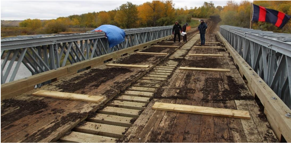
Figure 3.5 - Bridge deck with rough surface simulated by installed boards
