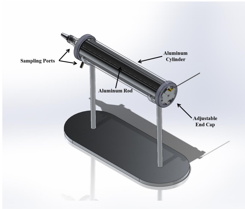
Figure 15: Mechanical 'sleeved forearm' apparatus used in the particulate transport benchmarking experimentation
