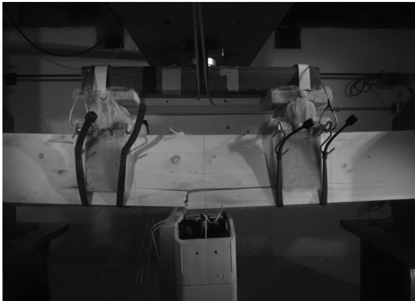
Figure 4-33: Footage from the high-speed phantom camera of DC2-178 at the beam's maximum deflection
