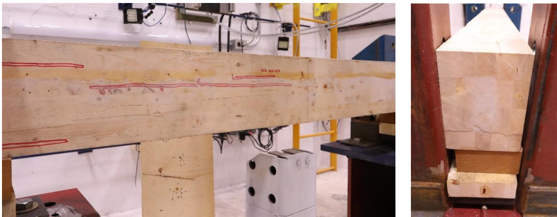
Figure 4-36: Shear and flexural failure in a dynamic cold temperature test specimen SN4-178
