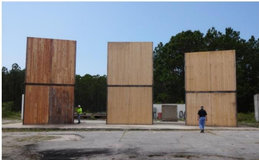
Figure 2-9: CLT structures pre-blast (Weaver et al. 2018)
