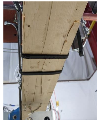
(c) Underside of specimen after failure
