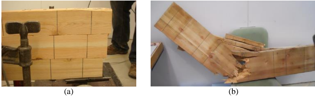
Figure 2-4: Specimen failure under four point bending: (a) Typical shear failure at 20°C (b) Typical tension failure at -40°C (Drake et al. 2015)
