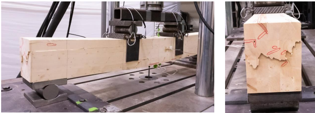
Figure 4-35: Combined shear and flexural failure in static normal temperature test specimen SN4-178
