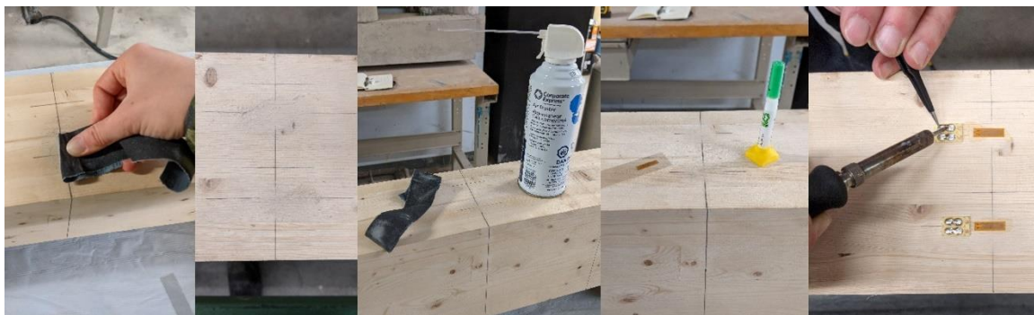
Figure 3-1: Preparation of the test sample for strain gauges. From left to right: sanding, sanded surface, compressed air, strain gauge and glue, soldering of tabs and leads
