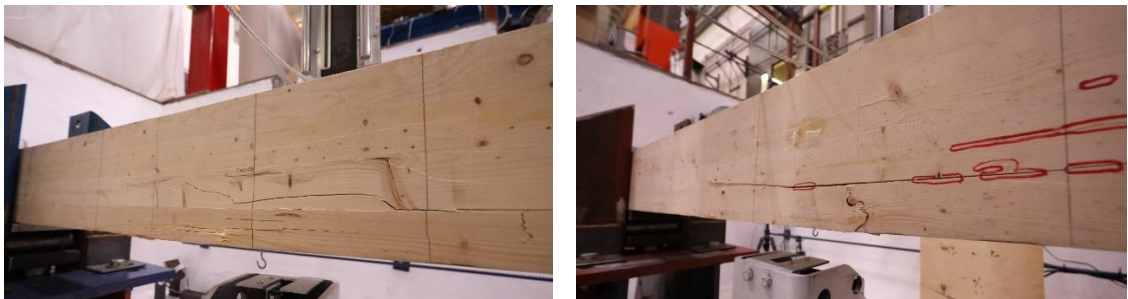
Figure 4-30: Failure of a dynamic normal temperature specimen, DN1-178 in the testing pit
