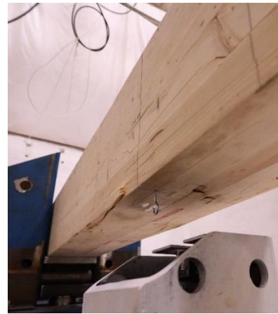
(c) Underside of specimen after failure
