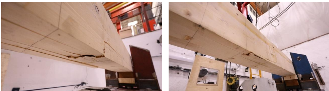
Figure 4-31: Failure of a dynamic cold temperature specimen, DC1-178 in the testing pit
