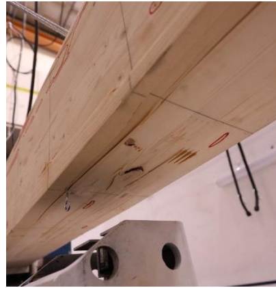
(c) Underside of specimen after failure
