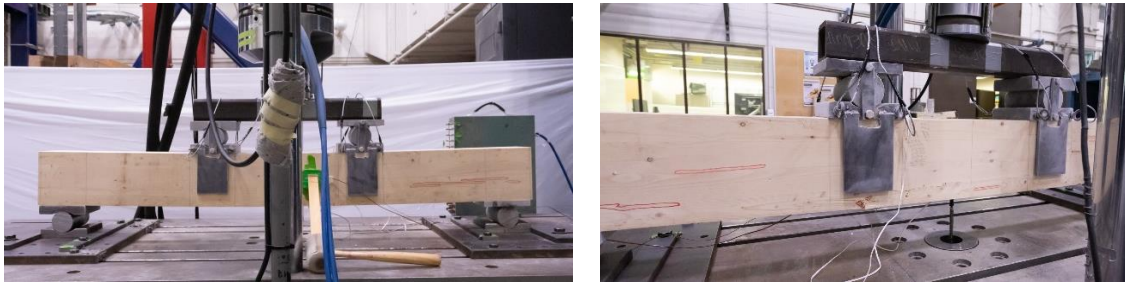
Figure 4-29: Failure of a static cold temperature specimen, SC1-178, within the testing apparatus
