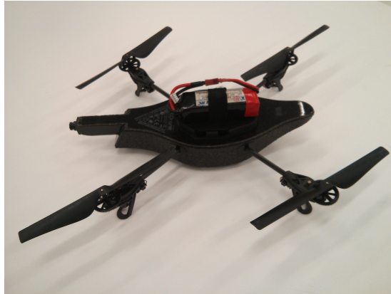
Figure 3.3: The AR.Drone modified battery holder (foam removed for illustration purposes)
