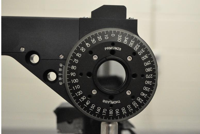
**Figure 3.6: Analyzer rotary stage with analyzer polaroid mounted. Note, the rotary stage has rotated the optical axis of the polariser to the  $90^\circ$  position.**
