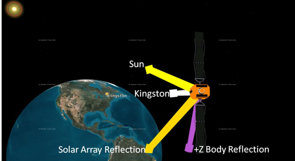
Figure 5.9: Solar array and +Z body specular reflection vectors on 8 August 2015.
