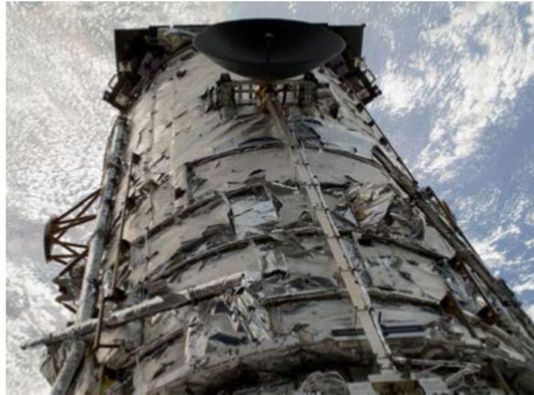
Figure 1.12: Space weathering damage to the Hubble Space Telescope [16].
