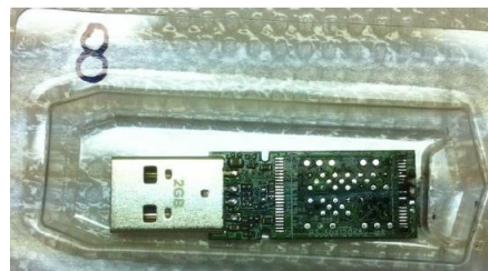
Figure A-5: Corroded USB Device
