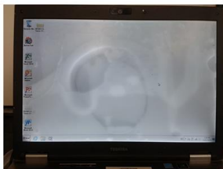
Left: Thin-Film Transistor screen 13 min after immersion in FK-5-1-12
