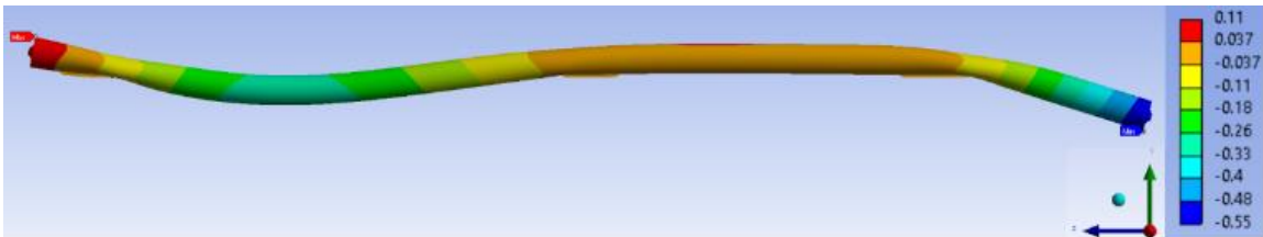
Figure 28: Vertical deformation of an Outer Fuel Element with End Flux Peaking Temperatures, Pellet Weight, Creep, and Free Endcaps (mm, 50X Magnification)
