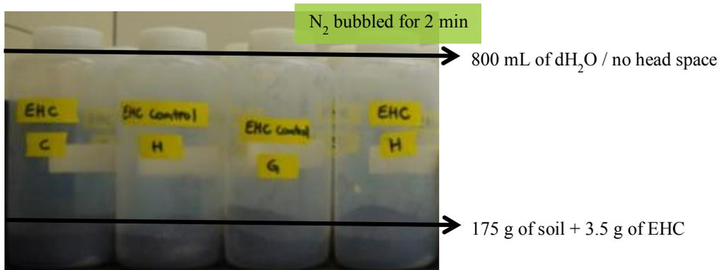
**Figure D-9.** A representation of the EHC experiment that simulated a groundwater environment at the RMC laboratory.
