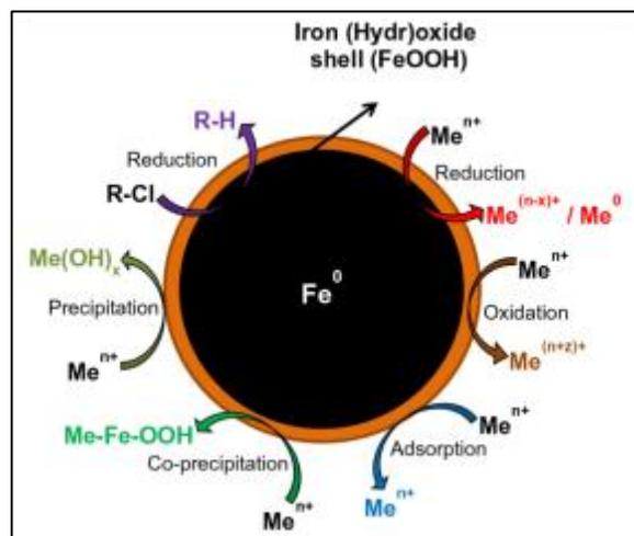
**Figure 2.5.** Core-shell structure of nZVI depicting various mechanisms for the removal of metals and chlorinated compounds (from O’Carroll *et al.* 2013).
