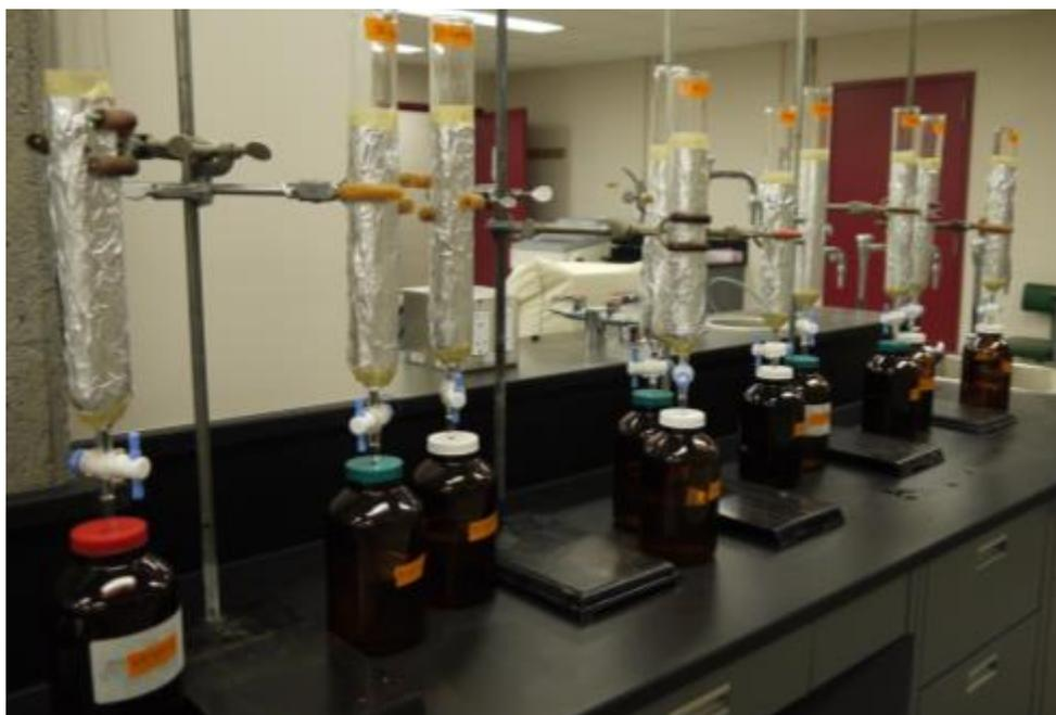
**Figure D-4.** The columns in the optimal HP $\beta$ CD concentration experiment at RMC.
