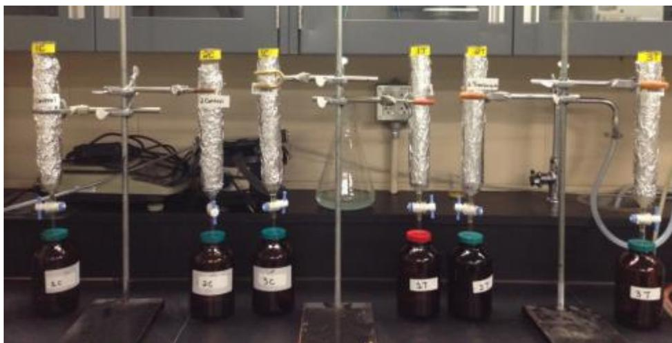
**Figure D-3.** The six columns in the microbial activity experiment at the phytoremediation laboratory at RMC.
