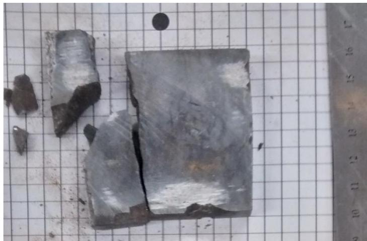
**Figure 5-22** First rock sample after damage in Test 0040 at 475 kPa
