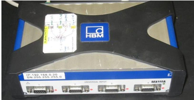
**Figure 4-19** Quantum X MX440A DAQ
