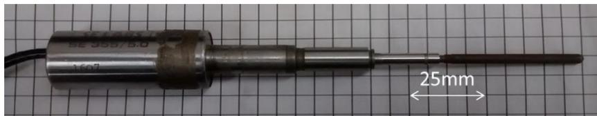
**Figure 4-14** SE Labs DCDT used for horizontal displacement
