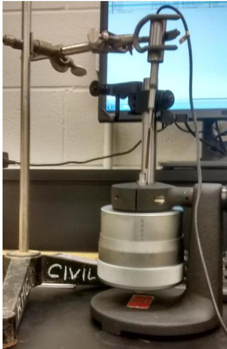
**Figure 4-16** Pedestal micrometer calibration set-up
