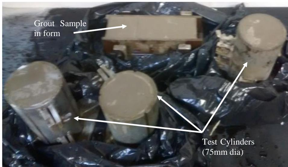
**Figure 3-10** Grout samples for both shear and compressive strength testing
