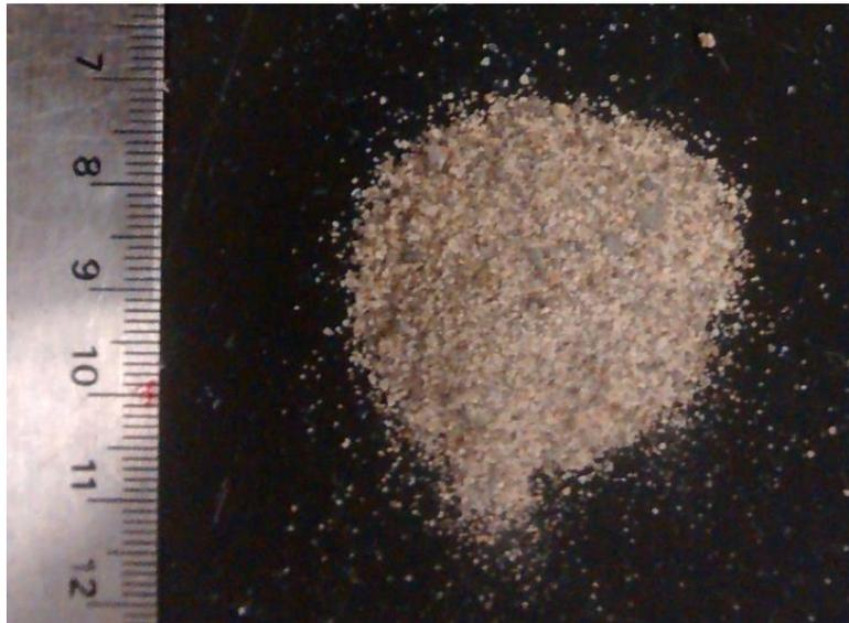
**Figure 3-4** Poorly graded Brighton Beach Sand
