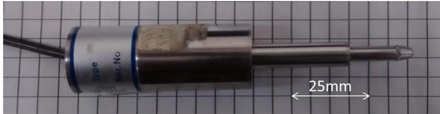
**Figure 4-12** RDP D2/200A DCDT used for vertical displacement
