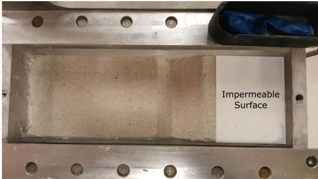
**Figure 33 Impervious Road Surfacing with Paraffin Wax**
