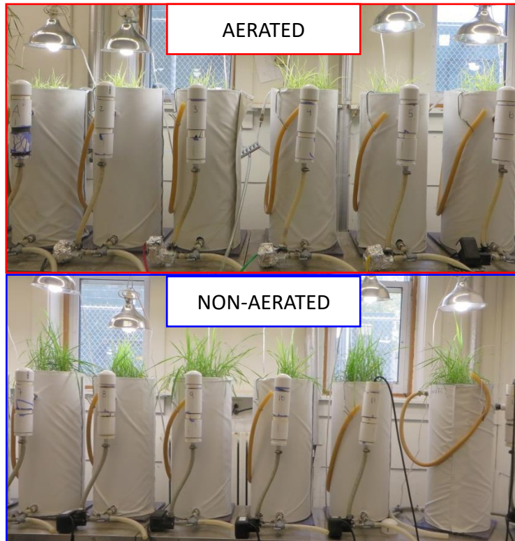
Figure 4.1: Mesocosm experimental design showing six aerated and six non-aerated CW mesocosms, planted with Phalaris arundinacea .
