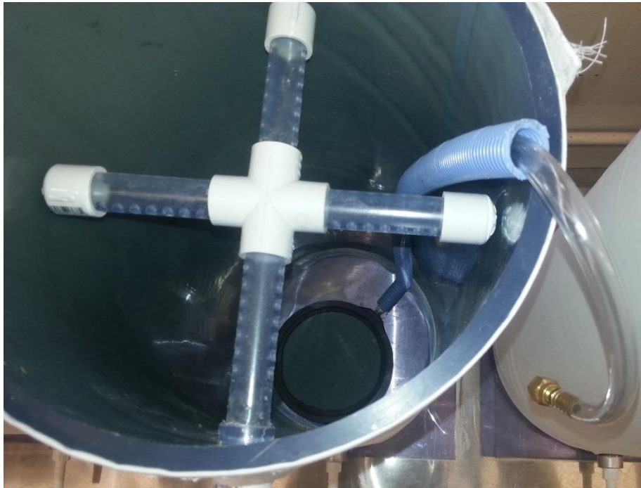
Figure 3.3: Image depicting the placement of an aeration stone within a mesocosm. The blue corrugated tubing surrounding the Nalgene tubing was used to prevent collapse from the weight of the substrate media.
