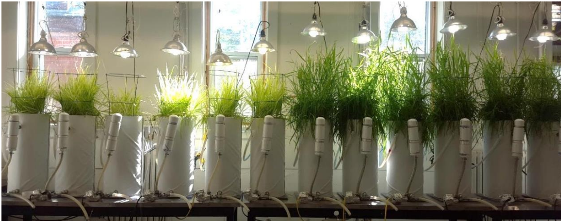
Figure 3.5: Laboratory mesocosm set up. The six aerated mesocosms are on the left with the six non-aerated mesocosms on the right. Plant lights were affixed approximately 6-12 inches above the maximum stem height of the plants and moved accordingly as the plants grew. This is a sample picture taken a few months after the start-up study experimental period.
