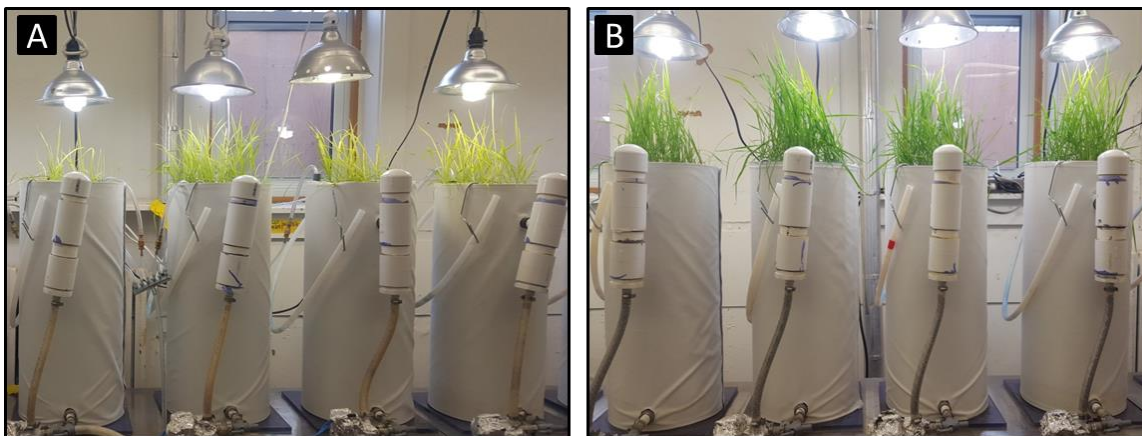
Figure 3.7: Sample image of plant growth in aerated (A) versus non-aerated (B) CW mesocosms. The addition of aeration is not favourable for the health and growth of Phalaris arundinacea causing the stems to be bleached relative to those grown in a non-aerated environment.
