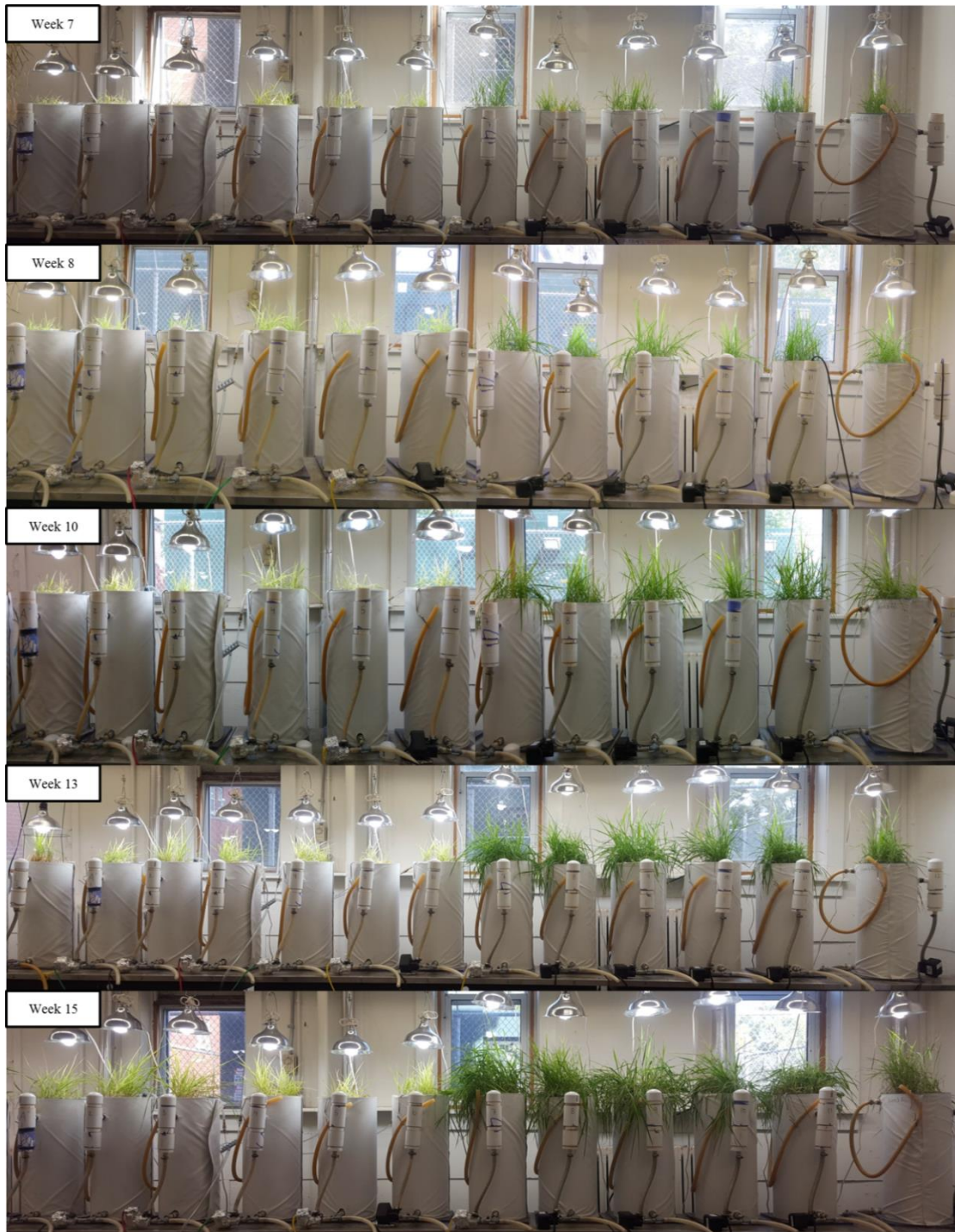
Figure 4.16: Plant growth progression in aerated (left six, light green) versus non-aerated (right six, dark green) constructed wetland mesocosms. Pictures are included from week 7, 8, 10, 13 and 15.
