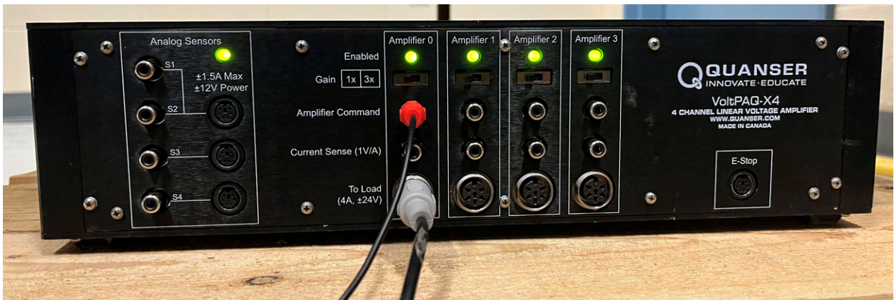
Figure 5.3: Amplifier Used to Power Motor
