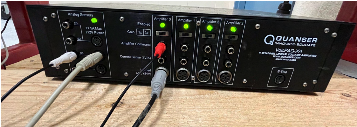
Figure 5.28: Amplifier Used to Power Motor and Flexcam Sensor
