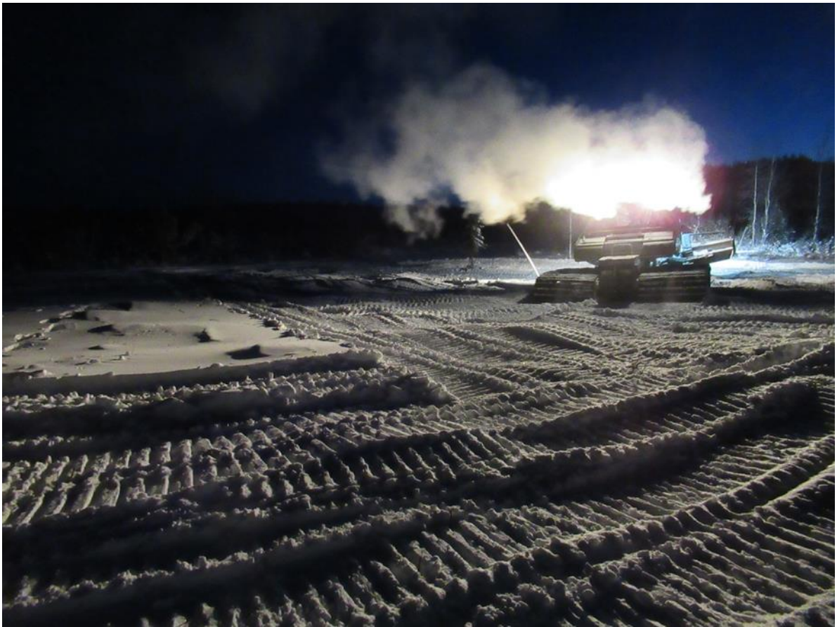
Figure 7: A picture of the field site undergoing snow compaction by driving a Sno-Cat over the site (Photo Credit: Alice Wilson & the Northwest Territories Geological Survey).
