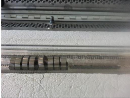
**Figure 13: Sealed ampoule with iodine capsule inside furnace before heating.**
