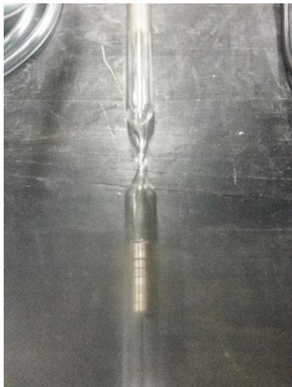
**Figure 11: Necked down glass ampoule.**
