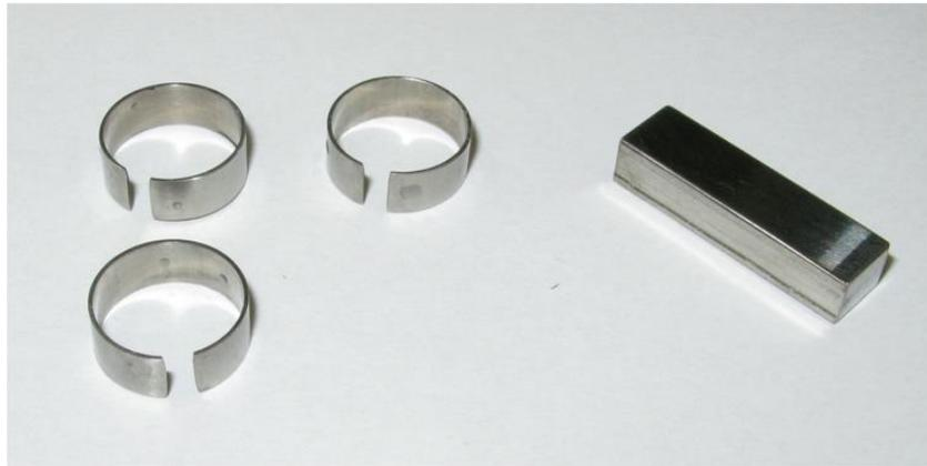
Figure 8: Zr-4 slotted ring samples and a Zr-4 static wedge.
