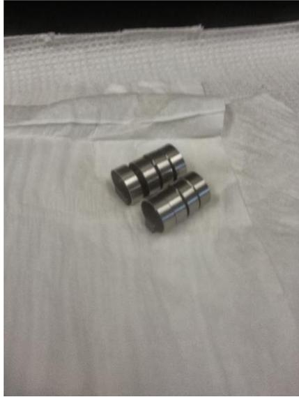
**Figure 9: Loaded slotted ring samples.**
