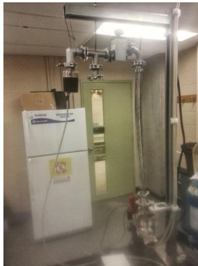
**Figure 12: Vacuum system for evacuating ampoules.**
