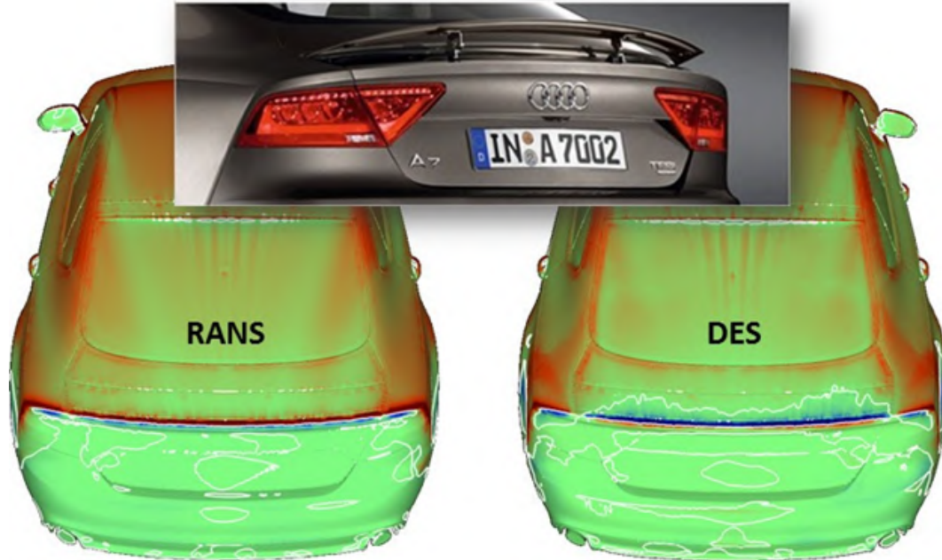
Figure 2.2: Differences in RANS vs. approximate DES surface sensitivities in the rear spoiler area, where red indicates moving the surface inwards to reduce drag and blue indicates moving the surface outwards to reduce drag [14].
