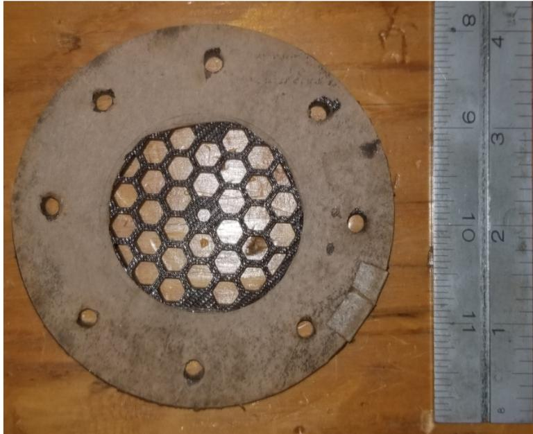
Figure 5.2: Restriction Screen used to Reduce Airflow at Combustion Chamber Inlet.
