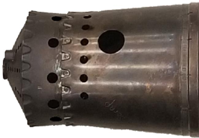
Figure 3.2: M250-C20B Combustion Liner.
