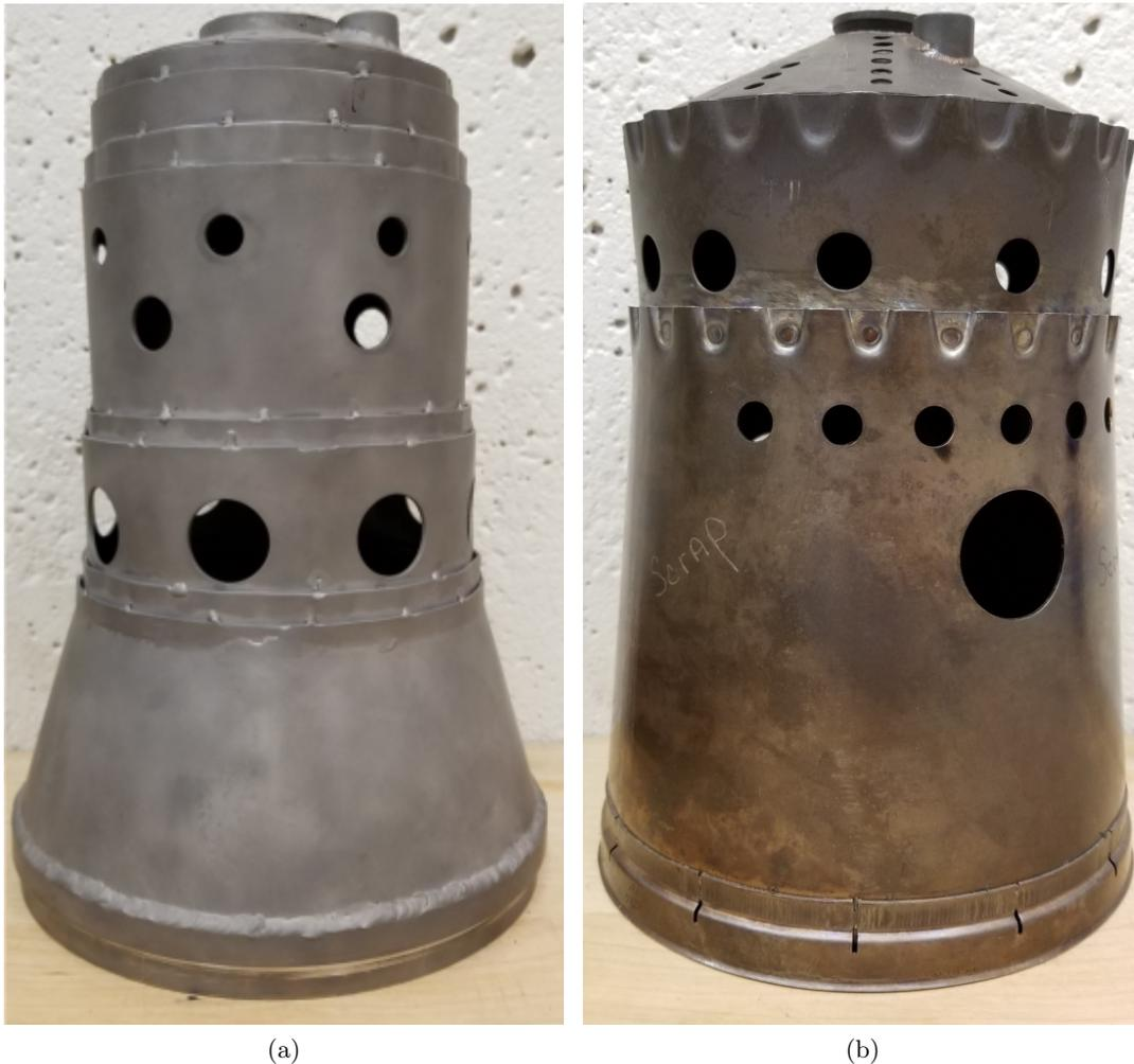
Figure 6.11: Hole Size and Placement (a) New Liner, (b) Original Liner.
