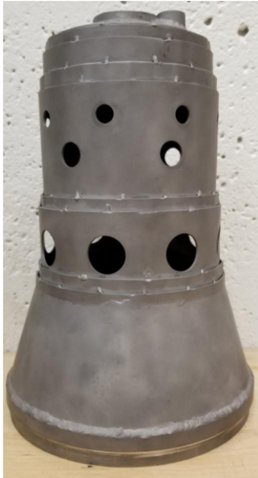
Figure 4.8: View of the Holes and Film Cooling Devices.
