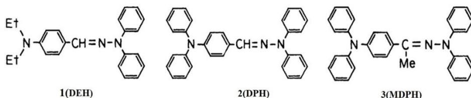
These families of molecular glasses are based on aryl hydrazones (**1-3**),<sup>13</sup> triphenylamine/triphenylbenzene (**4-7**),<sup>14,15</sup> and triphenylborane (**8-11**).<sup>16</sup> As the parent compounds readily crystallize, these glass-forming compounds are functionalized with conjugated arms which give the molecules their distinct star shapes
