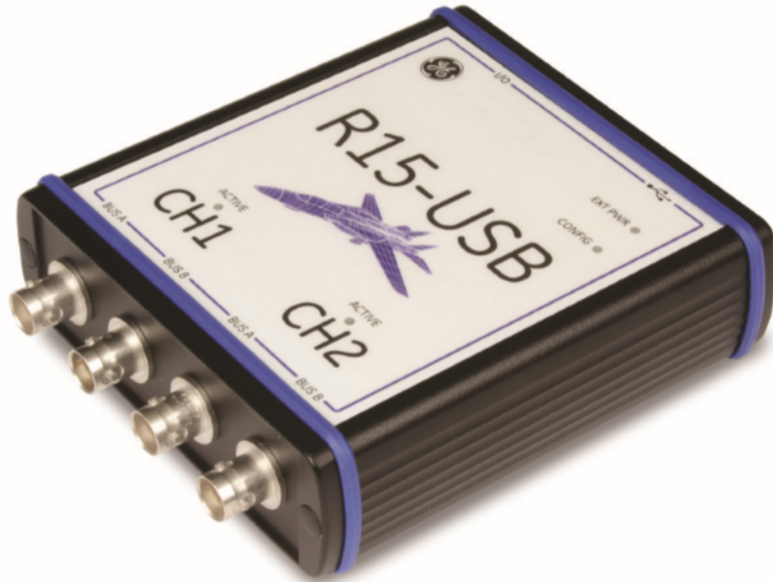
Figure 4.10: Abaco (formerly GE) R15-USB.
