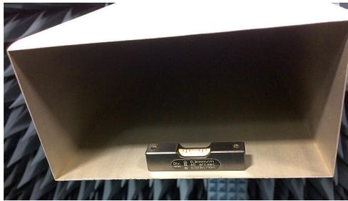
Figure 6.3: NSI ANT-WGP-1.12-1.7 probe alignment.
