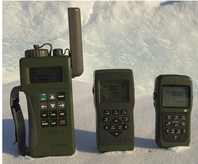
Figure A.2: Military handheld GPS receivers: PLGR+96, PLGR 3 and DAGR (© J. Lang, DRDC Ottawa, 2003).
