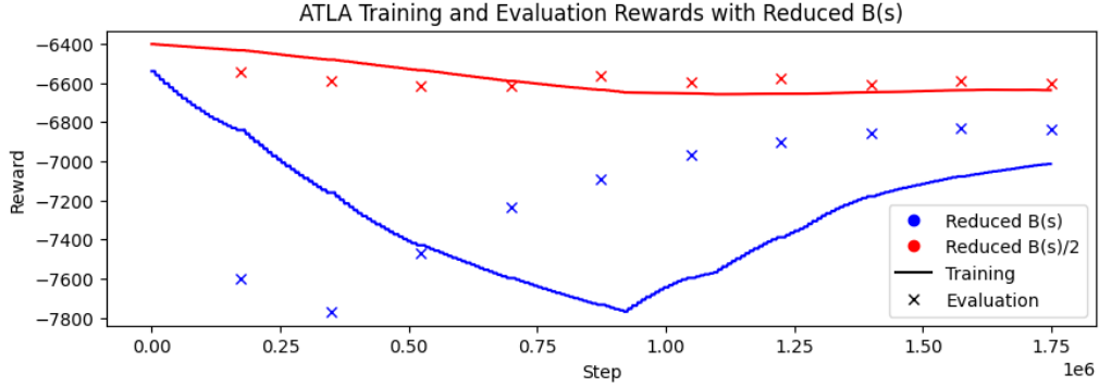
Figure 54: Line plot comparing the training curves for different adversarial budgets B(s) . The LA is a SAC and the agent a discrete PPO. The final evaluation rewards indicate that both agents reduce power consumption, however the attack using B(s)/2 does not have a significant effect on the agent. Reducing the adversarial budget produces more capable agents than those plotted in figure 53.
