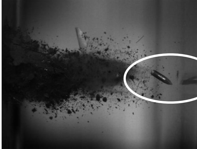
*Figure 3-24: Tumbling of the Penetrator at the Exit of Specimen UF4-60-2*
