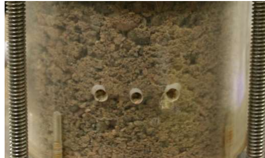
Figure 5.2.1: Dry SF-1 in the column showing segregation
