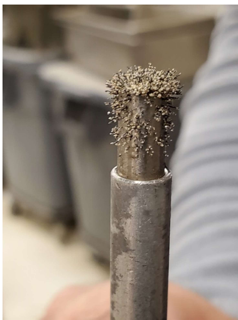
Figure 6.7.5: Magnetic fines on a magnet after being inserted into soil
