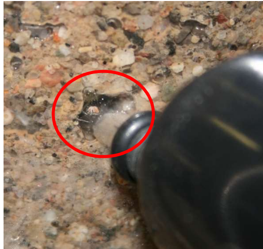
Figure 6.7.3: Soil Grains displacement during insertion
