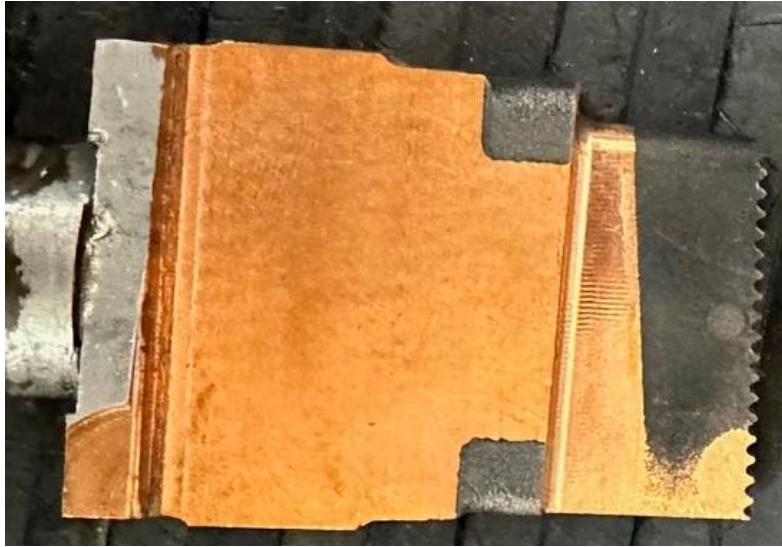
Figure 3.13: Electrode used for the modification of compressor blades
