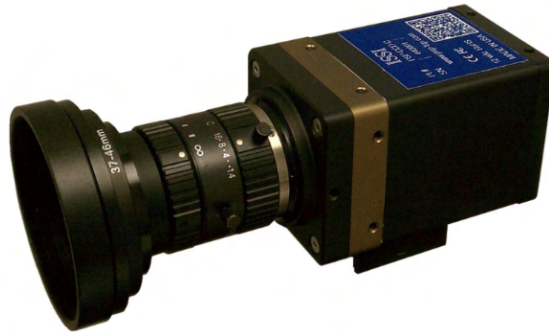
Figure 3.11: Image of PSP-CCD-C camera used for PSP [9]
