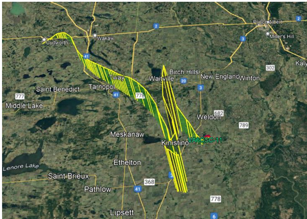
Figure 5.6 Flight path of the VHF relay balloon
