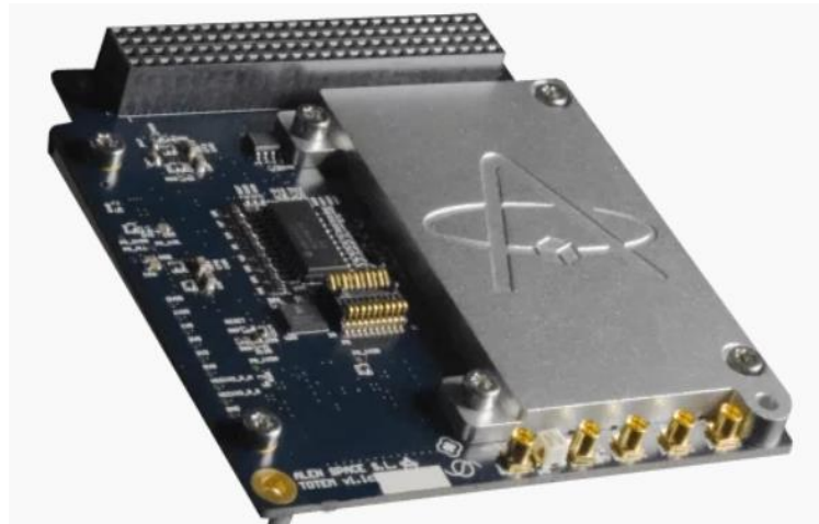
Figure 6.1 TOTEM SDR with wideband transceiver [120].
