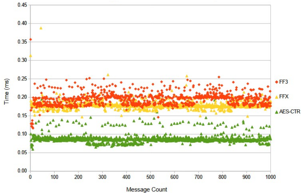
Figure 17: Encryption time with 0.5 s delay on the RP using all three FPE algorithms
