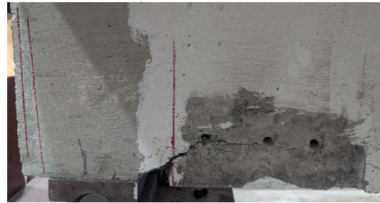
(b) After removal of the anchor
