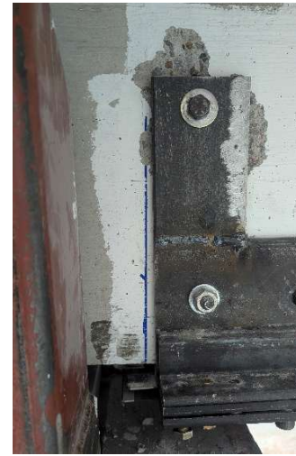
(b) Anchor on SB-2.2 after testing
