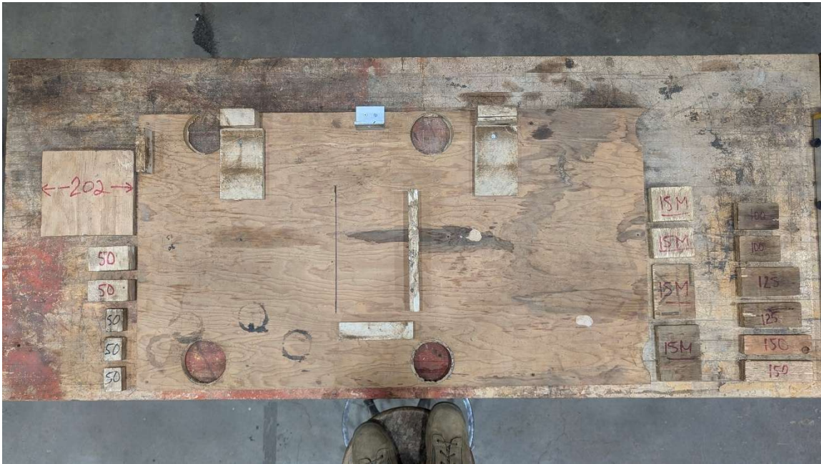
Figure A-2. Jigs for Reinforcement Bars Cages
