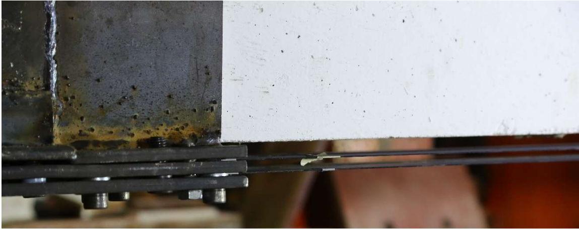
Figure 3-4. Close-up of CFRP Installed on SB-2.2
