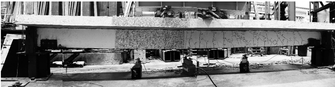
Figure 3-18. SB-2.1 double layer at failure
