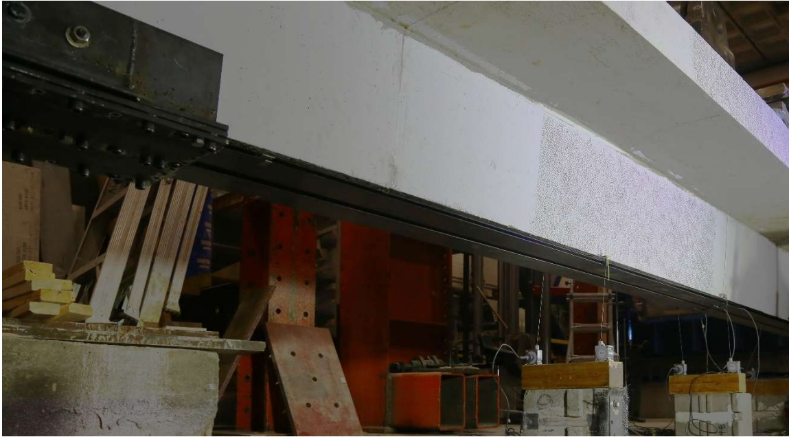
Figure 3-6. CFRP Installed on SB-2.2
