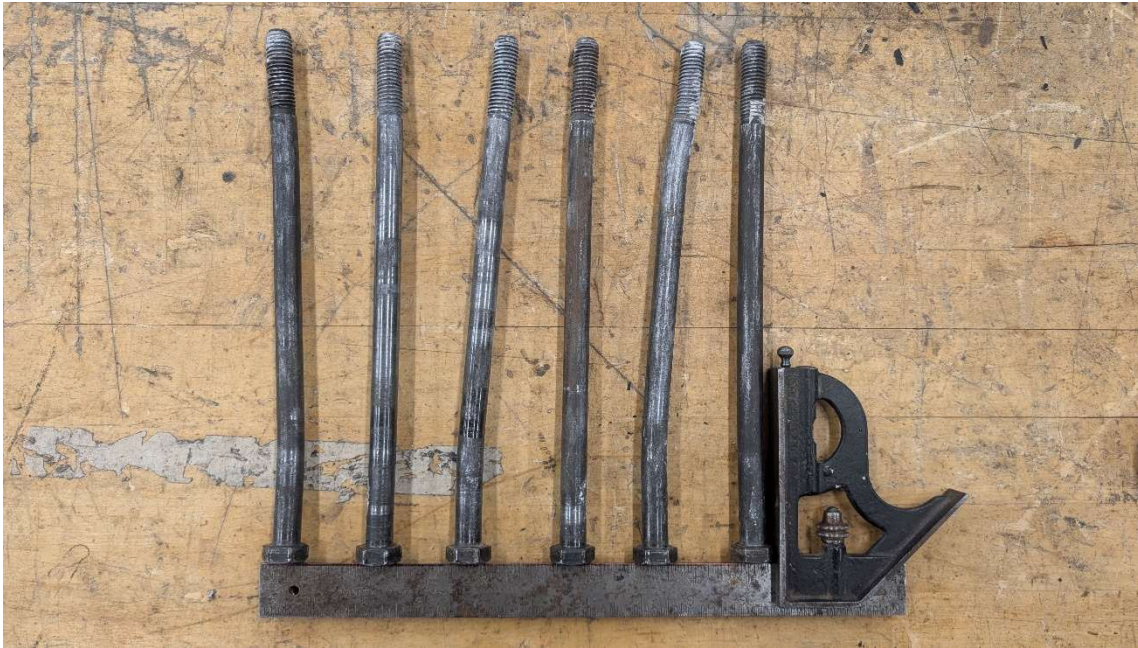
Figure A-5. Deformed Anchors' Bolts
