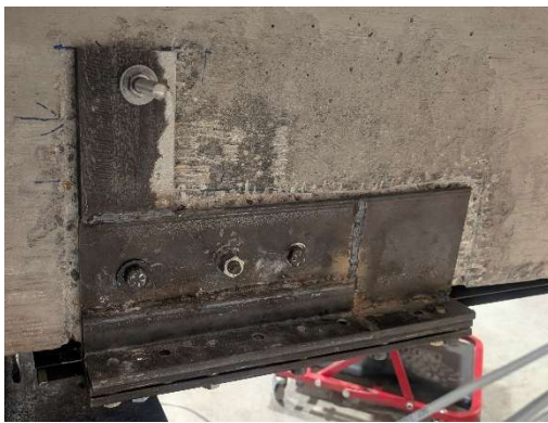
(a) Anchor Installed on SB-2.2
