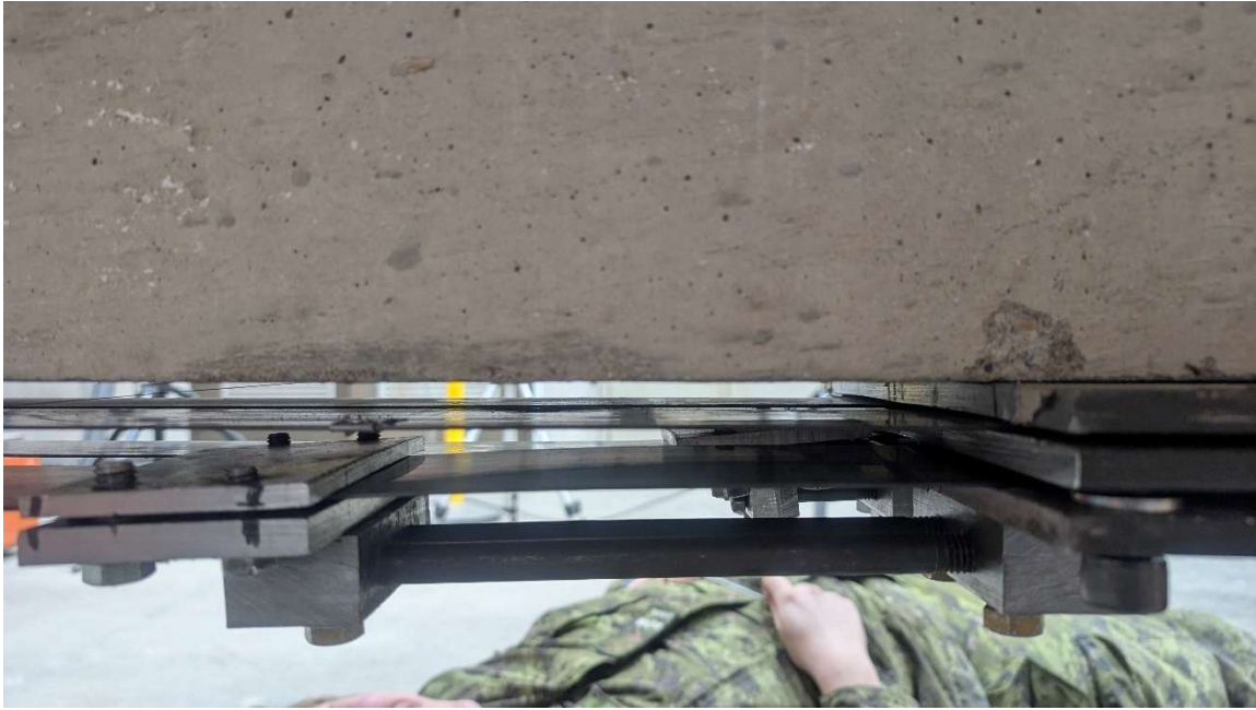
Figure A-6. Tensioning Device Twisting the Strap
