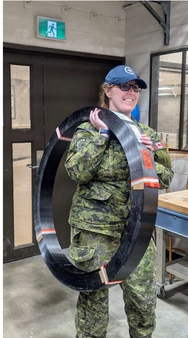
Figure A-4. Demonstration of Lightweight Property of the CFRP
