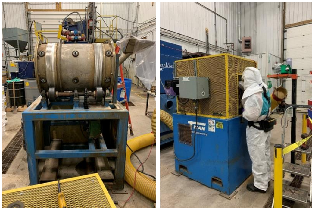
Figure 2-8: A Titan Process Equipment Ltd. custom process HBM with 267 L cylinder with and without the protective cage. Photo at right for sense of scale.
