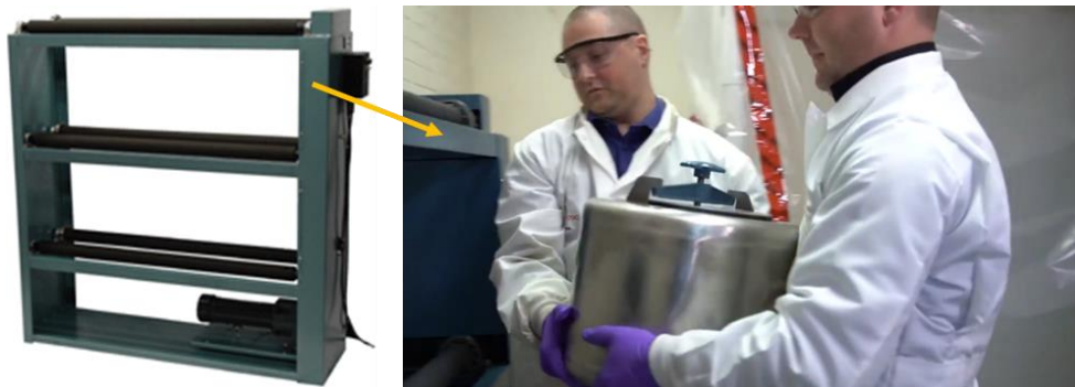
Figure 2-7: A U.S. Stoneware 3-tier long roll HBM (model #803DVM) with 25 L stainless steel cylinder. Photo at right for sense of scale.
