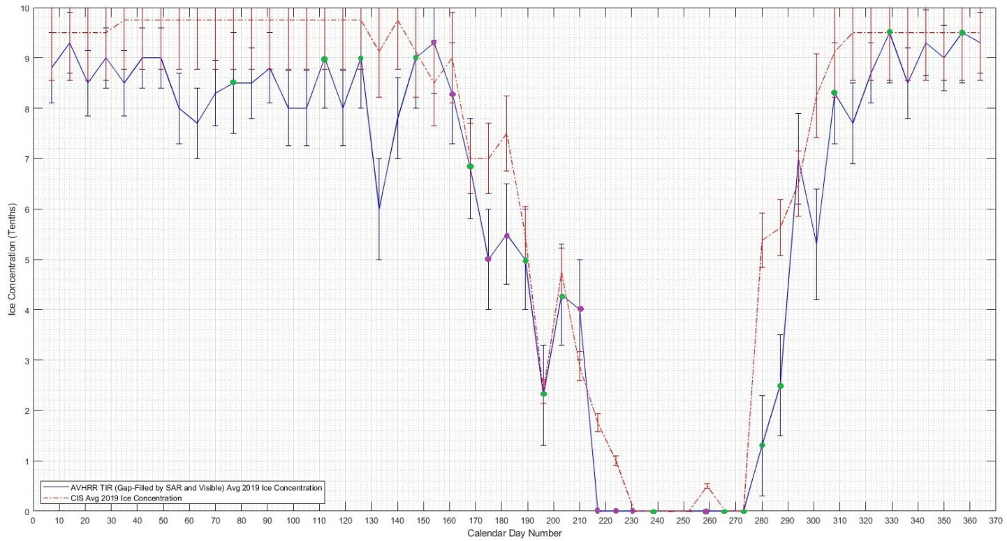
Figure 3.7: 2019 average IC results for Lancaster Sound using ACIC (gap-filled by SAR and AVHRR visible channel) and CIS ice charts. SAR used on calendar days 77, 112, 126, 147, 168, 189, 196, 203, 238, 266, 273, 280, 287, 308, 329, 357 (green dots). AVHRR visible channel used on calendar days 154, 161, 175, 182, 210, 217, 224, 231, 259 (purple dots). Days 245 and 252 had no data, so assumed as OW.
