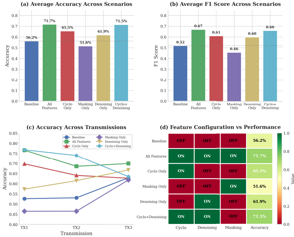
FIGURE 3. Ablation study performance comparison. (a) Average accuracy across evaluation scenarios for each configuration. (b) F1 score comparison showing consistent patterns with accuracy results. (c) Accuracy variation across UAV transmission instances (TX1–TX3 shown as representative subset; the full TX3–TX19 evaluation yields the reported 92.9% aggregate accuracy). (d) Feature configuration matrix summarizing the P1/P2/P3 combinations tested. The optimal configuration (P1+P2) achieves 71.5% accuracy with 1.47x computational overhead.
