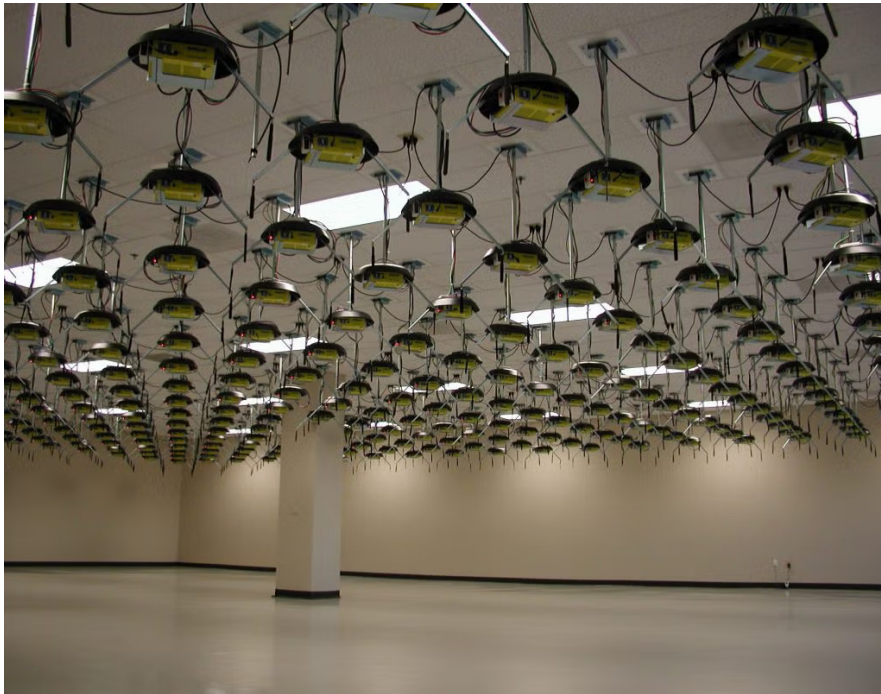
Figure 3.1: WiSIG experimental infrastructure showing Orbit testbed architecture with 20 \times 20 grid configuration and USRP receiver placement
