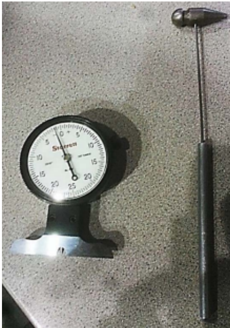
Figure 2.8: A tap tester (right) and a depth gauge (left) are typically used in evaluating BVID damage in aluminum honeycomb sandwich panels [24].
