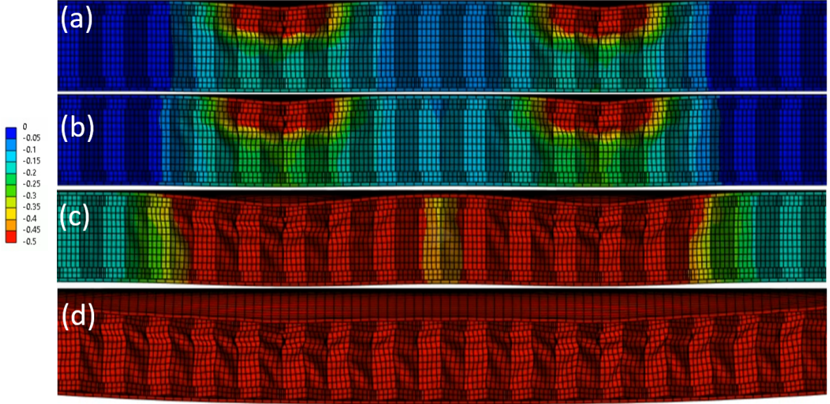
Figure 5.11: Z Deformation(mm) of a 45mm center-to-center spacing at (a) beginning of Stage 2, (b) panel yield, (c) at peak force, and (d) panel failure.
