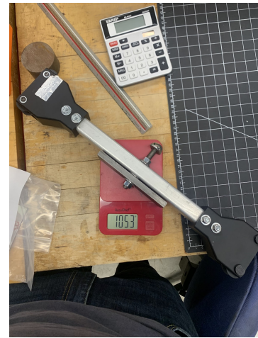
(b) Drop tower section that is in free fall during indentation shown being weighted.
