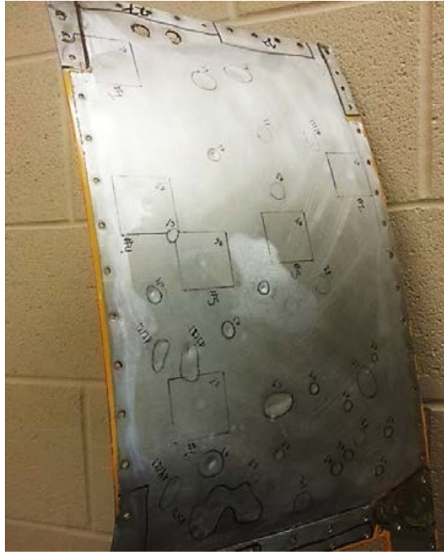
Figure 1.4: An aluminum honeycomb panel with multiple low-velocity impact damage sites that was retired from a CH-146 Griffon helicopter.
