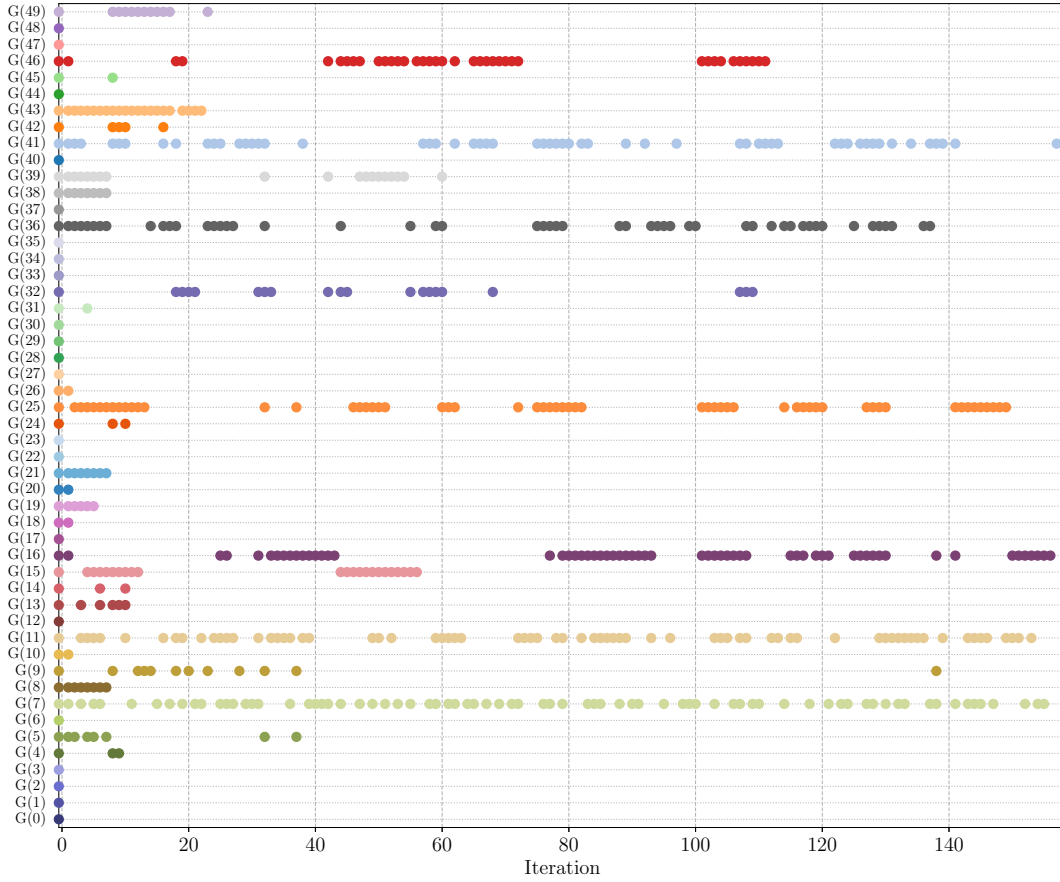
Figure H.18: Scatter of constraints not meeting the tolerance threshold for the relaxed constraints for the nacelle configuration, with payload.
