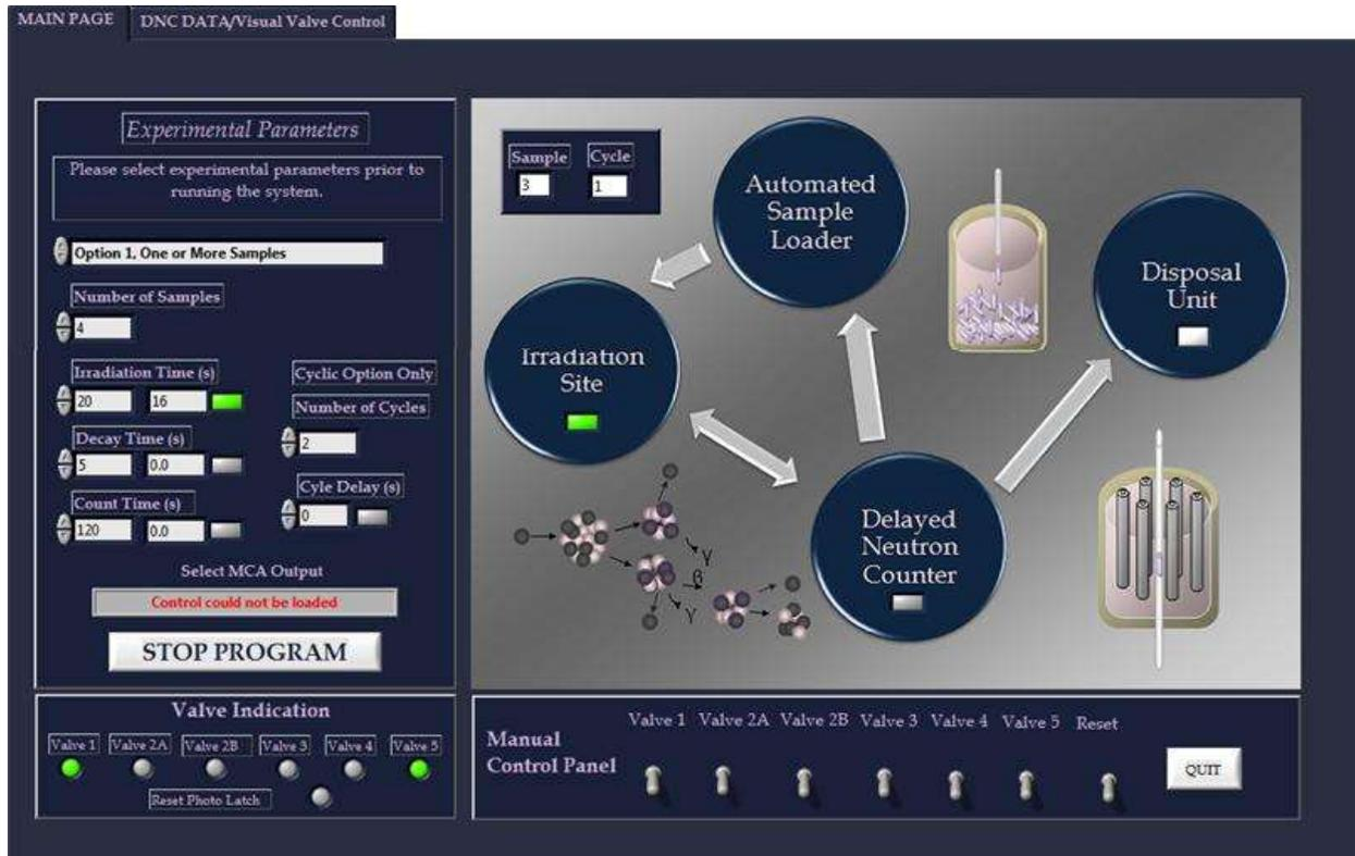
Figure 4-1: Delayed Neutron Counting Graphical User Interface
