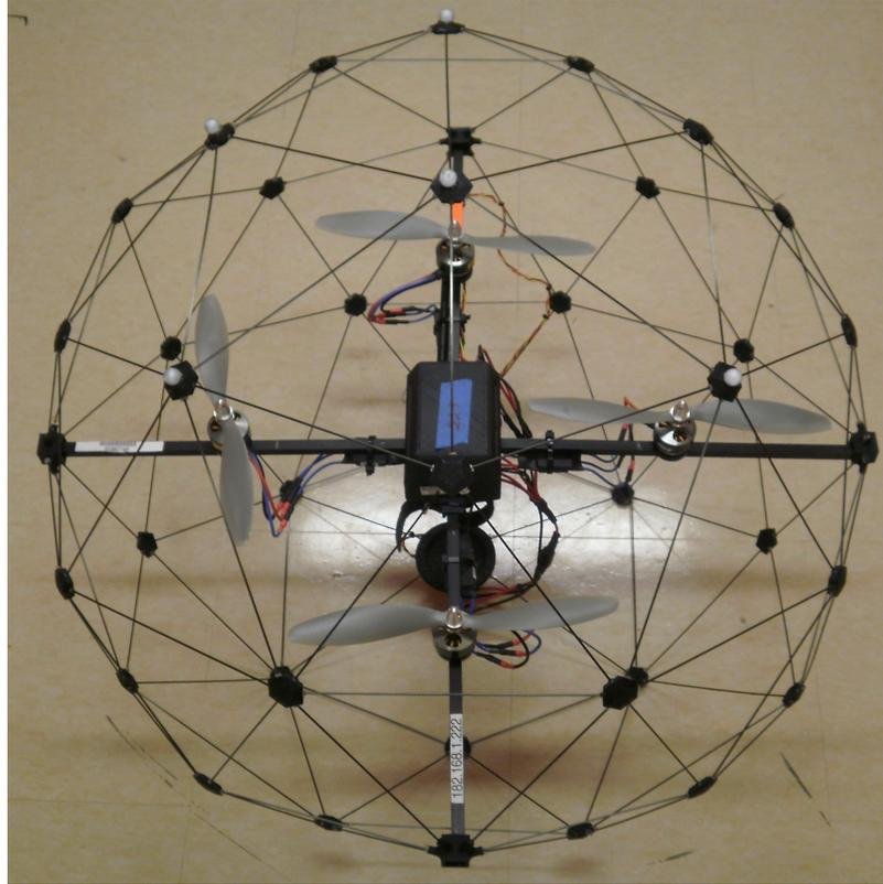
Figure 2.5: Qball-X4 quadrotor aircraft. The frame around the motors and CPU assembly is strictly for equipment safety.
