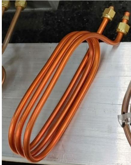
Figure 70: A custom designed induction coil for scanning operations.
