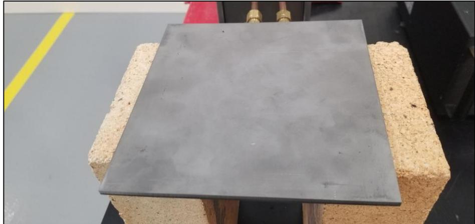
**Figure 2:** Sample located over the induction coil.
