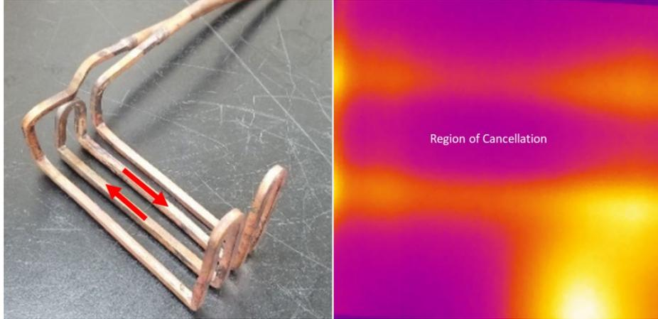
Figure 83: Cancellation effect observed with the channel coil. The red arrows show the opposing flow on alternating current.
