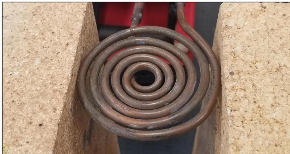
**Figure 1:** Induction coil used in the experiment.
