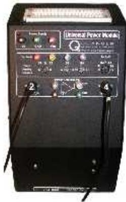
Figure 7.8 Yaw motor voltage amplifier (UPM-1503) [61]
