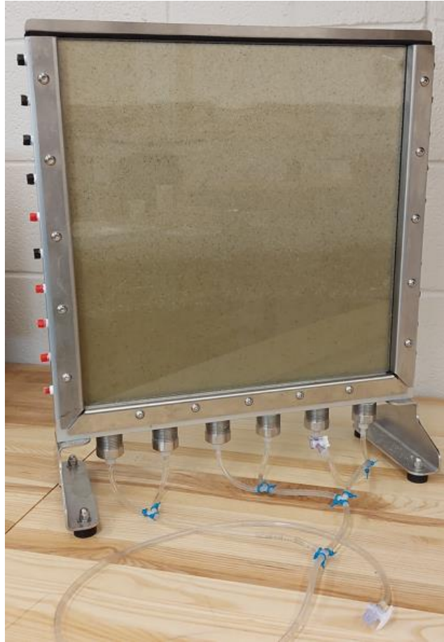
FIGURE 2.2: Flow cell image showing the cell frame, glass panels, bottom ports, and flexible transparent tubes. Each port is topped with a water-wet net filter.
